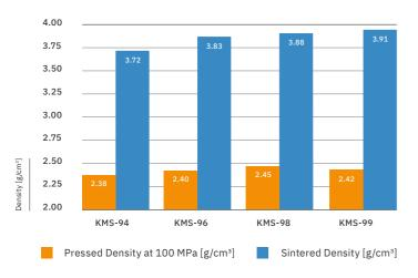
The density data at pressed and sintered stages proves the ability of the KMS granules to produce high performance components while remaining cost effective.
